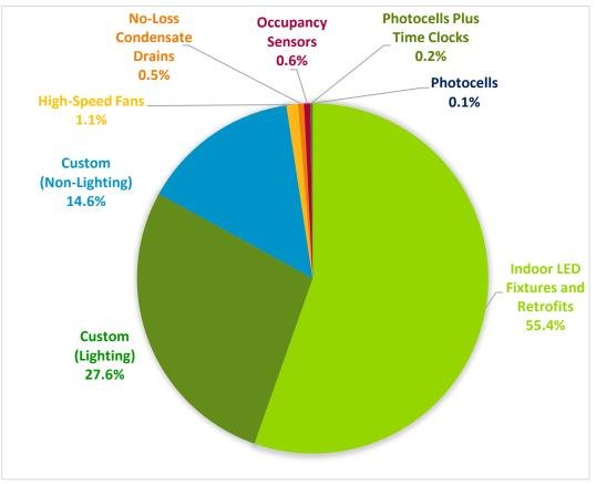
Figure 5-1. Verified Net Savings by Measure – Electric
