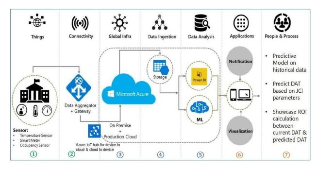
Figure 1: Optimized air handler system architecture. Green (1-2) represents layers located on-site at the Art Institute. Blue (3-5) represents layers located in the Azure Cloud, and orange (6-7) represents the user-facing layers accessible via the internet.
